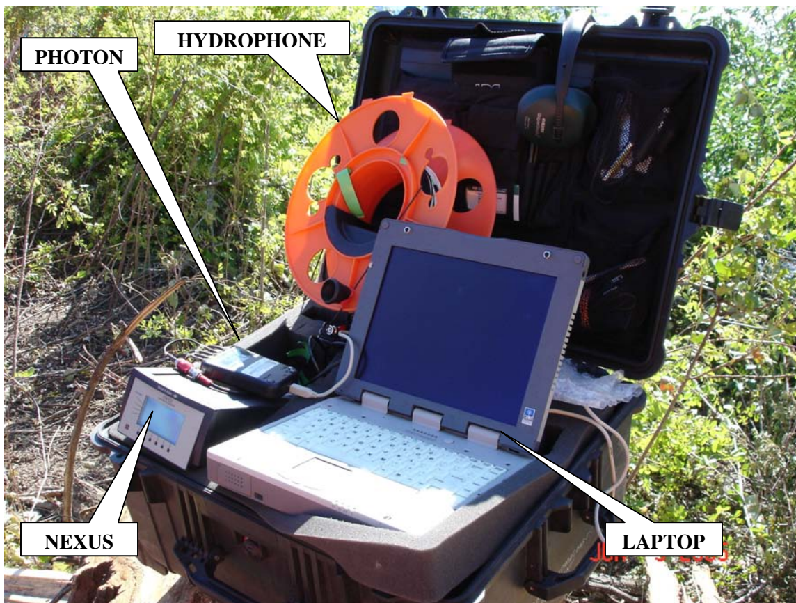
Figure 4: Underwater Sound Level Measurement Equipment
