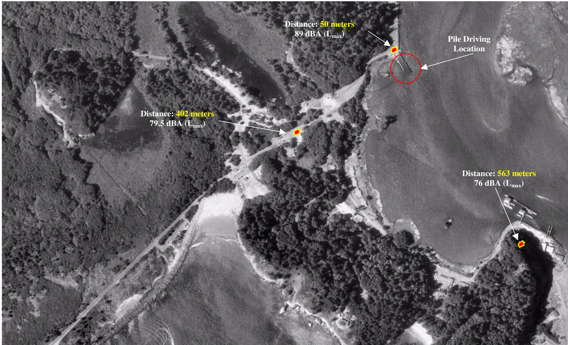
Figure 11: Airborne measurement locations (☀) with A-weighted maximum values.
